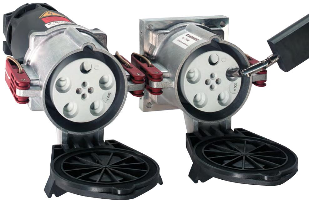
The heavy-duty series plugs and sockets extend the currently standardized plugs and sockets according to EN 60309-2 by rated currents from 160 A to 600 A as well as rated voltages of up to 1000 V. They are built in accordance with the following standards: IEC / EN IEC 60309-1.
