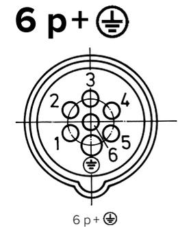
to IEC 60309-1, EN IEC 60309-1, DIN EN IEC 60309-1 (VDE 0623-1), DUO-Interlock to IEC 60309-4, EN IEC 60309-4, DIN EN IEC 60309-4 (VDE 0623-3).
